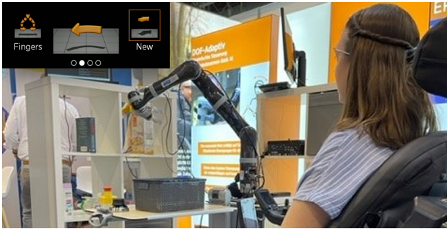
Fig. 1: Study apparatus at the trade fair, illustrating the placement of user, table, and shelf, as well as the UI visualized on the smart glasses (top left)
