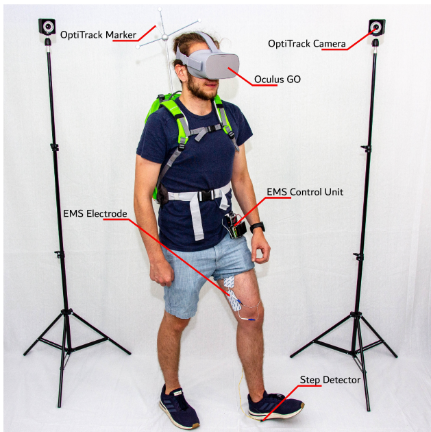
Figure 2: The Infinite Walking setup including cameras and markers for tracking, EMS Control Unit and Electrodes for actuating, Step Detector for properly timed actuation, and Oculus GO for displaying the VR scene. (Staged scene)
