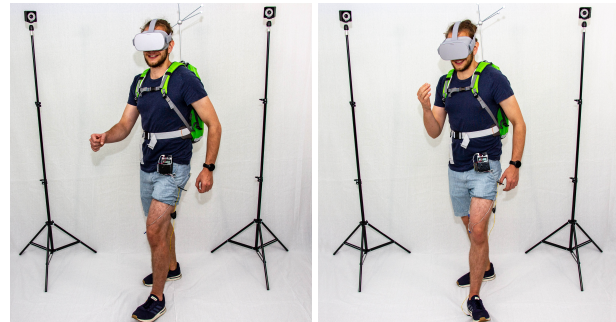
Figure 1: Left, the user walking in VR on a straight path. Right, the user's leg is rotated via EMS to the left. Now the user walks on a circle. (Staged scene)
