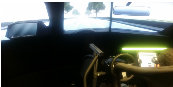
Figure 1: Experiment setup with the feedback bar mounted on top of the tablet showing the non-driving task.
