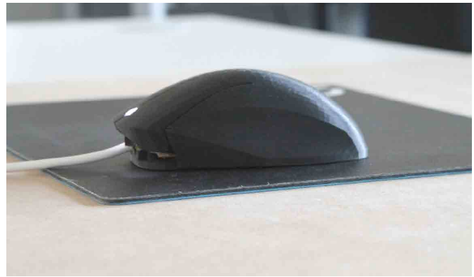
Figure 2. Rendered cross section (l.) and photo (r.) of the 3D printed mouse. The mouse includes an optical mouse sensor, a motor for button actuation, two neodymium magnets at the front and two at the back. A LED is placed between both mouse buttons for external tracking. The robot head holds three magnets at the front, and three at the back.
