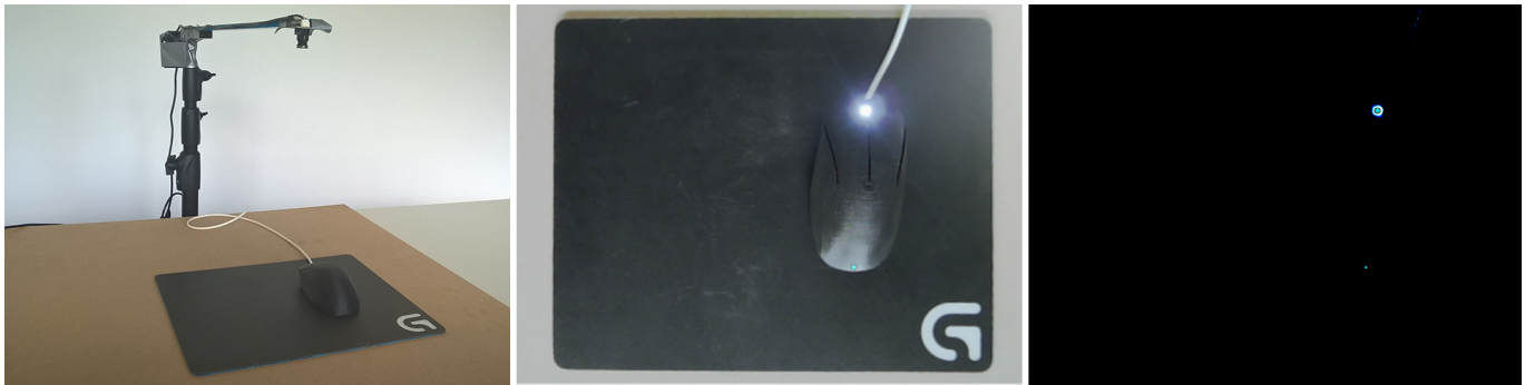
Figure 4. Camera setup (l.), distortion removed camera view (m.), and mouse LED position detection pass (r.)
