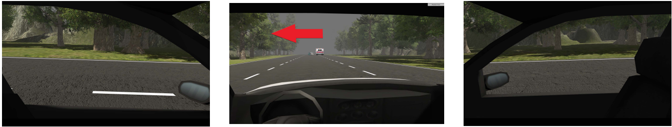
Figure 3: The autonomous vehicle driving on a 3-lane highway road, when it encounters an accident blocking the right and the middle lanes. A visual TOR is issued, indicating the free open lane for crossing.
