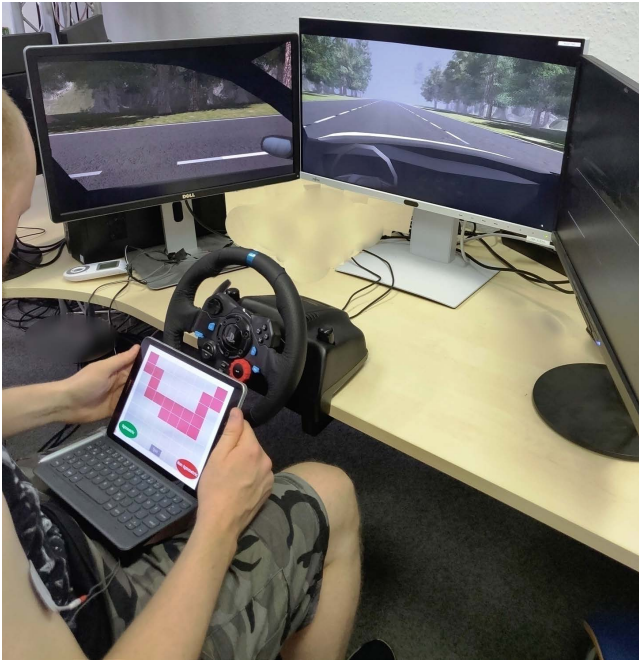
Figure 2: The final setup of the simulation used in the study. We presented the view on three displays (i.e., one for the front and two for the side), along with a Logitech G29 driving wheel. The non-driving task is displayed in a tablet placed on the driver’s lap.
