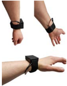
(a) Our hardware prototype being able to deliver warmth or coldness, respectively at the exterior and interior side of the wrist.
