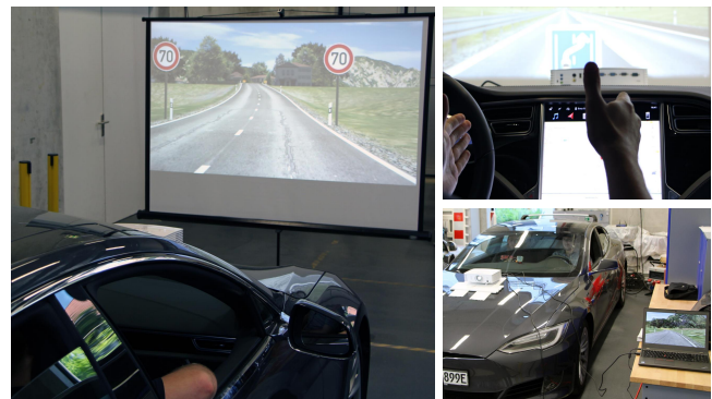
Figure 3: Experimental setup of the user study. We used a Tesla P60 and a large projection screen showing the driving maneuvers.
