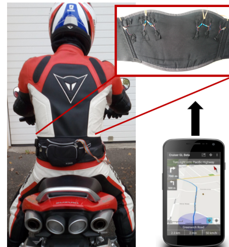
Figure 1. The MOVING system consists of a kidney belt with 12 integrated vibration motors controlled through a mobile phone application.
